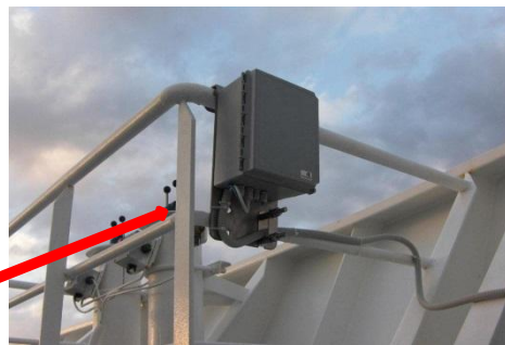
Telemetry box installed on bow open deck.
