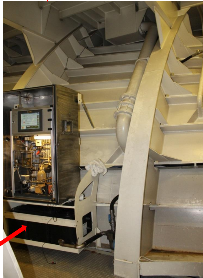
Telemetry box installed on bow open deck.
